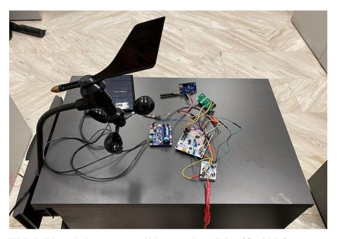
This is the "Maestro" telemetry system, which supports the prediction of fire risk in forest areas based on measurements of weather conditions, which are collected by wireless networks (nodes) of sensors, placed in the forest areas.
